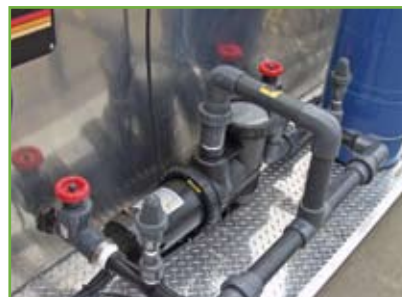
Mazzei® venturi air injection system sustains beneficial aerobic microbes, while destroying odor causing anaerobic bacteria.
